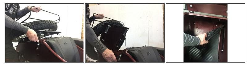
• Open trunk and remove contents to gain access to the sidecar trunk hinge mounting hardware.
