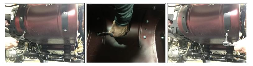
Use a 13mm tool inside and 5mm hex key outside to remove the four (4) lower sidecar trunk hinge bolts, nuts and washers.
